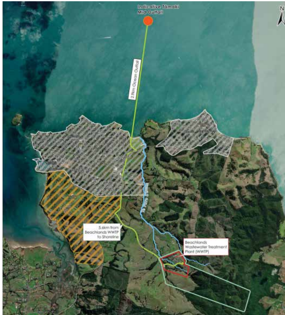
Map showing Watercare's option 4ae, which proposes piping treated wastewater via Te Puru to an outlet 2.9km offshore in the Hauraki Gulf/Tikapa Moana. Image / watercare.co.nz .
